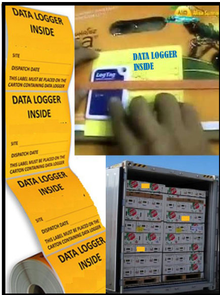
Figure 35. Illustration showing sample labeling and marking of boxes with data loggers inside. (Source: J. Saenz – Adapted from published online photos.)
