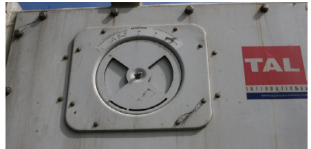
Figure 4. Picture illustrating manual fresh air exchange within a reefer container. (Source: PEB Commodities, Inc.)
