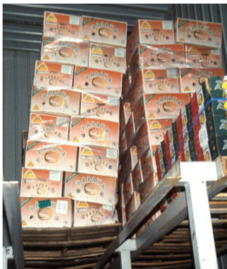
Figure 24. Failure of the bottom cartons due to poor construction or improper stacking. (Source: S. Sargent)
