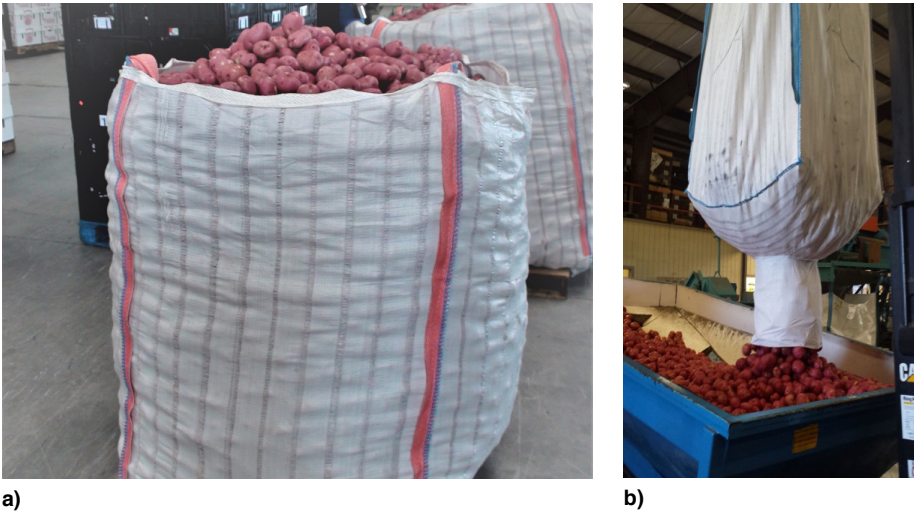
Figure 26. Potatoes a) stored in a super sack and, b) being unloaded onto the packing line. (Source: S. Sargent)
