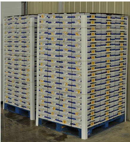
Figure 27. Palletized flats of blueberries with horizontal strapping and corner boards. (Source: A. Berry)
