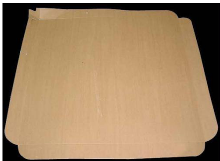
Figure 22. A slip sheet fabricated from fiberboard. (Source: J.K. Brecht)
