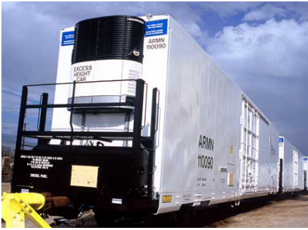
Figure 11. External view of refrigerated railcars. (Source: UPRR)
