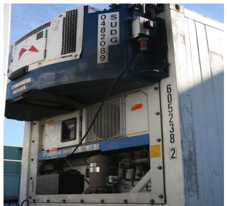
Figure 5. Clip-on gen set mounted to a refrigerated container. (Source: PEB Commodities, Inc.)
