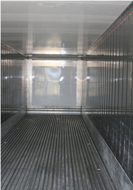
Figure 3. Interior view of a refrigerated container showing corrugated sidewalls, ‘T’ bar floor, return air register, and front bulkhead. (Source: PEB Commodities, Inc.)
