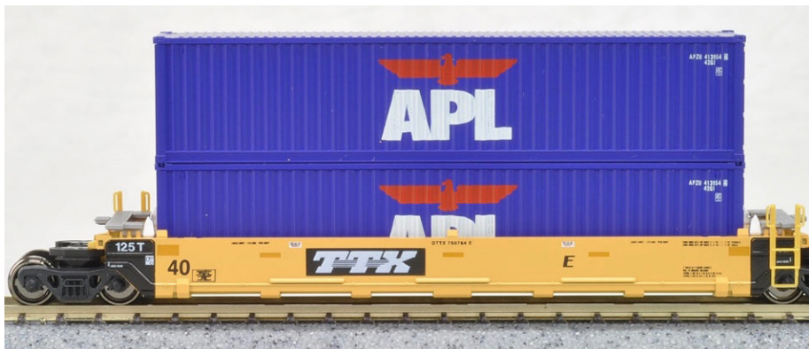
Figure 7. Reefer containers double-stacked on a rail stack car. (Source: American President Lines)
