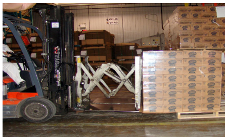
Figure 23. Stacked load on a slip sheet being pulled onto specialized forklift tines for transfer. (Source: Thida Sathorn Co.)
