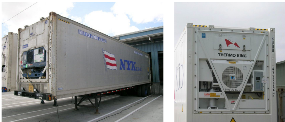
Figure 2. External views of refrigerated containers showing an integral refrigeration unit attached to an insulated container (box) and a chassis. (Source: PEB Commodities, Inc.)
