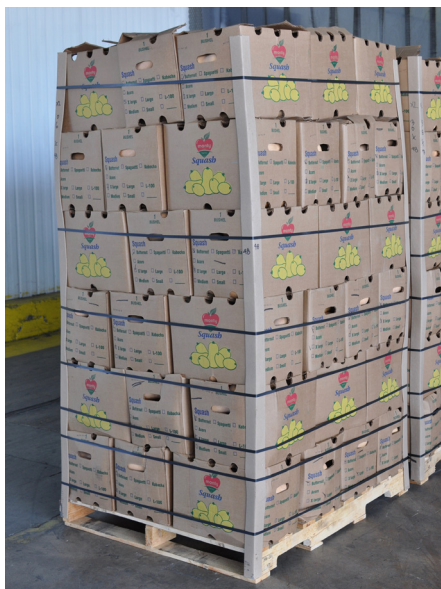
Figure 25. Cartons with vent holes designed to align when cross-stacked to allow both horizontal (top-air) and vertical (bottom-air) air flow during transport. (Source: J.K. Brecht)
