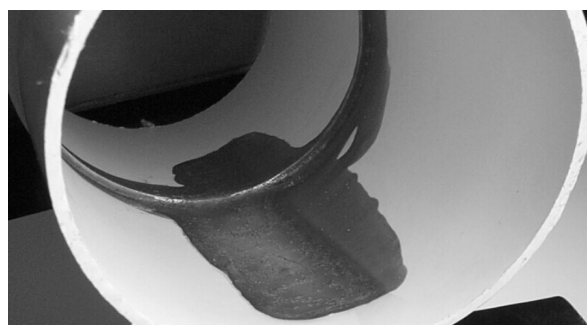
Figure 5. Excess cement used in PVC pipe joint resulting in softened pipe walls.
