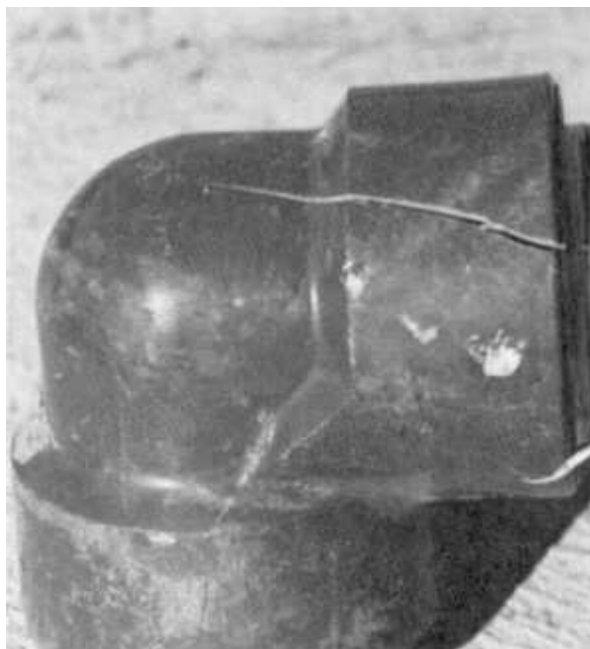
Figure 4. Example of threaded PVC fitting failure due to over-tightening (reprinted with permission from Bliesner, 1987).
