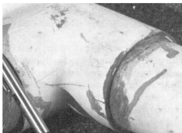
Figure 2. Example of long-term pressure failure in PVC pipe (reprinted with permission from Bliesner, 1987).
