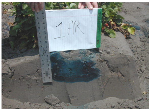
Figure 1. Cross section of beds after 1 hour of irrigation with drip tape that has 4-inch emitter spacing and a flow rate of 32 gal/100 ft/hr. Credits: J.R. Duval 2002
