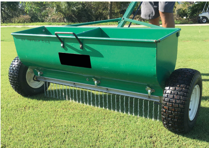
Figure 3. Drop spreaders distribute product uniformly between the wheels. Credits: Travis Shaddox, UF/IFAS
