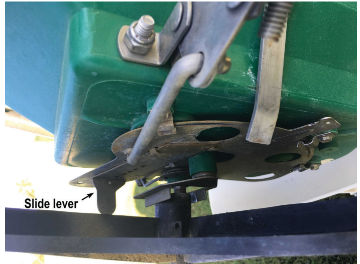
Figure 4. The slide lever on rotary spreaders can be adjusted so that the fertilizer is spread uniformly on both sides. Credits: Travis Shaddox, UF/IFAS
