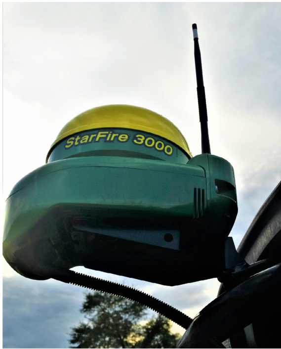
Figure 10. StarFire™ 3000 GNSS receiver and antenna mounted near the top of the cab of a John Deere 9770 STS. Credits: Rebecca Barocco, UF/IFAS
