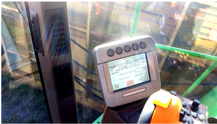
Figure 13. GreenStar™ 3 CommandCenter™ used for general combine controls and entry of calibration information on the John Deere 9770 STS.
