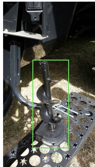
Figure 6. Small auger (inside green rectangle) for moisture sensor removed from cylinder container. Credits: Rebecca Barocco, UF/IFAS
