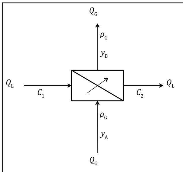
**Figure 5.** Blood oxygenator labeled with variables used in Eq. (3). Arrow in the center indicates oxygen mass transfer across membrane, which may be calculated using Eqs. (1) and (2) for the liquid side and gas side, respectively.
