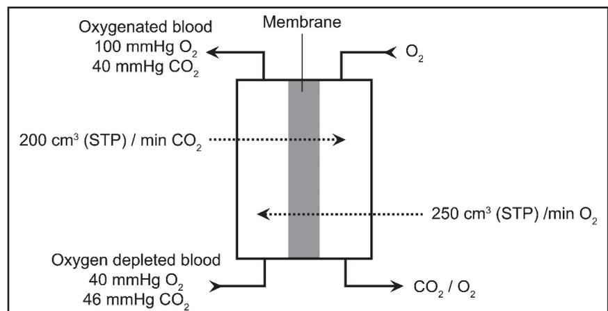
**Figure 3.** Membrane with gas transfer and concentration (partial pressures) values. As in the lungs, carbon dioxide is not completely removed to prevent alkalosis.<sup>[18]</sup>
