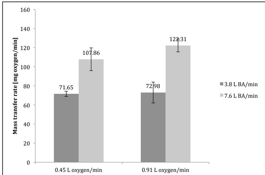
**Figure 7.** Mass transfer rates for all four operating conditions listed in Table 3 showing standard error of mean values. Each value is an average of gas side and liquid side mass transfer rates based on three trials. Error bars are standard error. The overlapping standard error bars allow students to conclude that the difference between means is significant, and therefore the oxygen flow rate does not have an effect on the mass transfer rate under these conditions.
