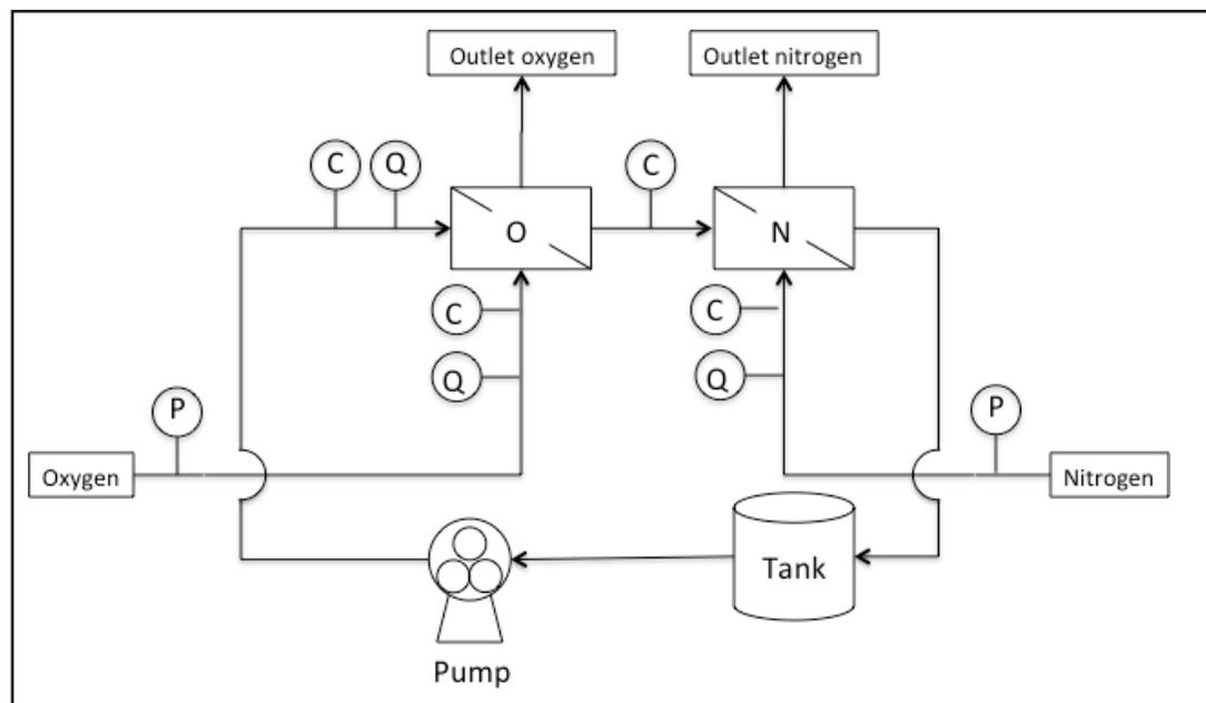
**Figure 4.** The blood oxygenator testing system showing the two hollow fiber membrane modules used for gas exchange (Module O oxygenates the blood analog; Module N deoxygenates the blood analog). Concentration (C) measurements are taken at the inlet and the outlet of each hollow fiber membrane module. Gas pressure (P) is measured on the oxygen and nitrogen inlet streams, and liquid flow rate (Q) is measured on the blood analog inlet stream.
