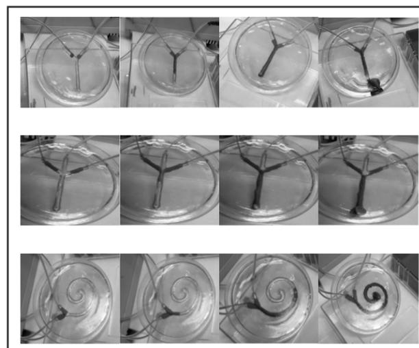
**Figure 2.** Fluid mixing on different gelatin chips. Red food color, milk, and blue food color were used for better visualization, as shown in different grayscale shades. The channel cross section was 3 mm by 2 mm (W x H).
