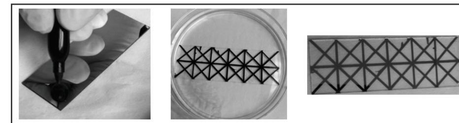
**Figure 4.** Copper electrode fabrication. The desired design was first drawn on a copper-coated glass slide with a permanent marker. Unwanted copper was etched away in a 3:1 mixture of 3%  $\text{H}_2\text{O}_2$  and 10 M HCl. To reveal the final copper electrodes, the permanent ink was washed away with acetone.
