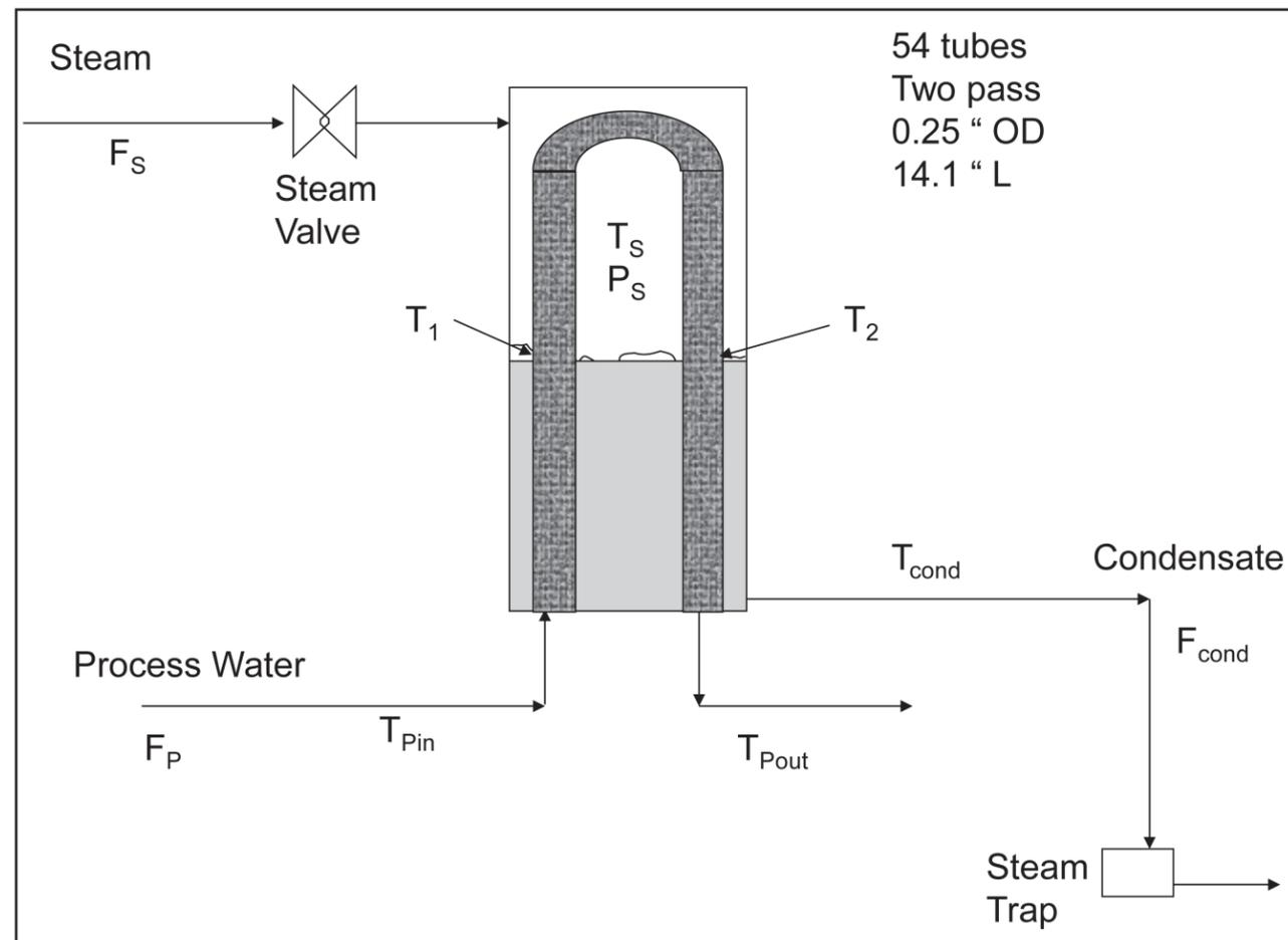
Figure 2. Flooded heater.
