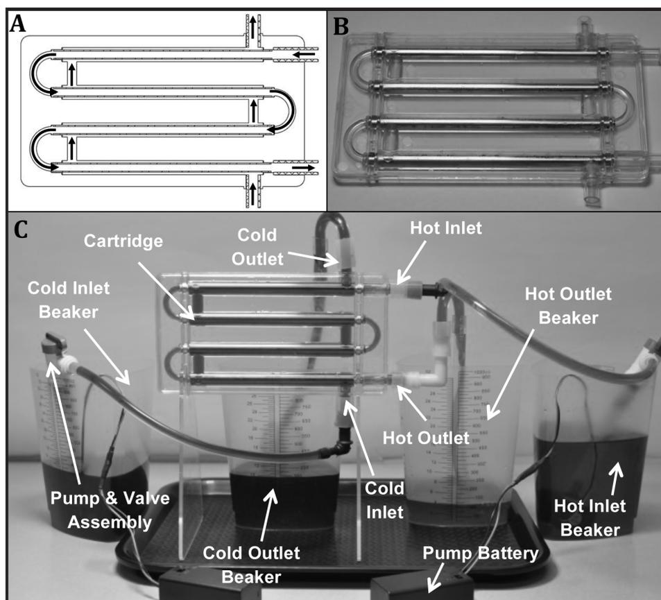
**Figure 1.** A) Simple schematic of a double-pipe heat exchanger LCDLM cartridge with arrows showing counter-current flow pattern, B) photograph of cartridge, and C) experimental setup for flow rate and temperature measurement with pumps in beakers connected to module via tubing and fittings.
