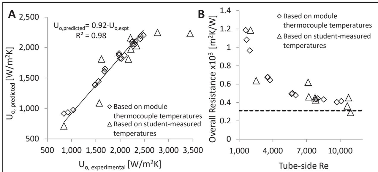
**Figure 4.** A) Predicted versus experimental overall heat transfer coefficient using thermocouple temperatures collected at module inlets and outlets or student-measured beaker temperatures, and B) experimental overall resistance versus the tube-side Reynolds number. The dashed line on (B) indicates the predicted sum of the annular and wall resistance, an asymptote reached at very high Re numbers.
