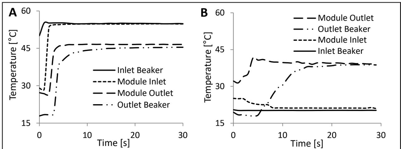
**Figure 2.** A) Hot-side temperature profiles for the inlet and outlet streams for fully open valve settings, and B) cold-side temperature profiles for inlet and outlet streams for a cold-water flow rate reduced to 6 mL/s.
