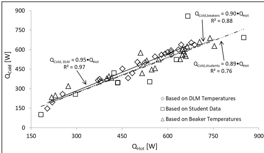
**Figure 3.** Hot- and cold-side heat duties calculated using temperatures collected via thermocouples at module inlets and outlets and in beakers, and by student groups or individual students using handheld thermometers.
