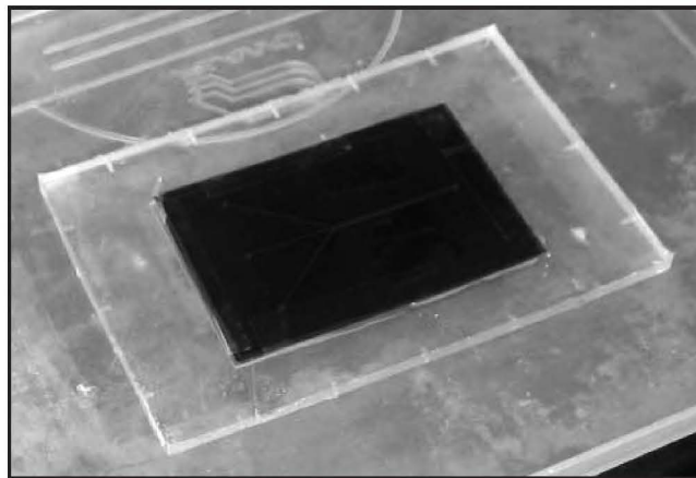
Figure 3. Mask added to glass slide on top of the PDMS frame containing optical adhesive.
