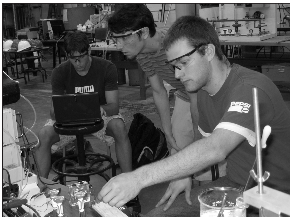
Figure 1. Chem-E-Car team testing the electrical performance of their fuel cell.
