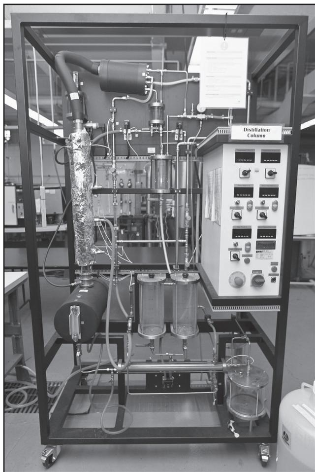
*A Distillation Unit in the Unit Operations II Laboratory (CENG 0420).*
