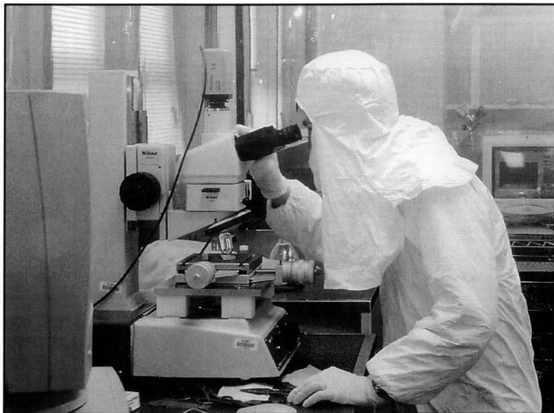
◀ Doctoral student Nitin Kumar prepares atomic force microscope for observations of the molecular surface topology of a silicon wafer modified by a molecular self-assembly technique.
