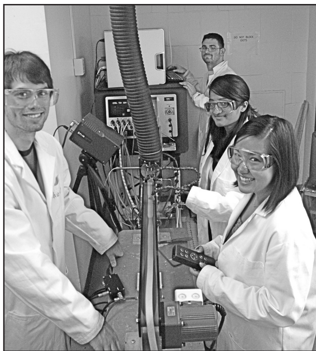
Figure 2. Students extruding Lexan ® (polycarbonate) with a ribbon die while following the solidification on the conveyor belt using an infrared camera.
