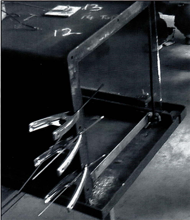
Figure 3. Incense sticks are placed to assist the observation of the behavior of air currents moving in and out of the opening.
