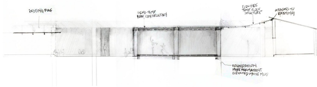
Figure 6. Cross section through exterior courtyard space proposed a raised ground and roof condition. This allows for a protected dancing space. May be temporarily used during the rainy season. © Ana McIntosh
